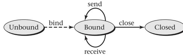
Figure 9.4: This state diagram shows the life cycle of datagram sockets used for sending or receiving UDP datagrams. In the Java API, the class `java.net.DatagramSocket` is used for this purpose, and binding happens automatically as part of the constructor.
