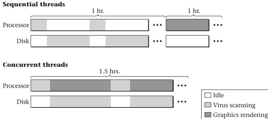
Figure 2.6: Overlapping processor-intensive and disk-intensive activities
