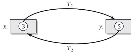
Figure 5.12: If transactions release each read lock as soon as they are done reading the corresponding object, the execution may not be serializable. For example, two transactions could swap  $x$  and  $y$ 's values, as shown here.
