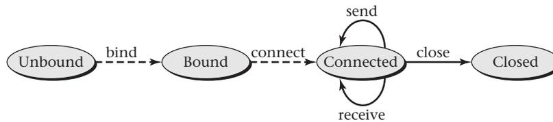
Figure 9.5: This state diagram shows the life cycle of client-side stream sockets used to initiate TCP connections. In the Java API, the class `java.net.Socket` is used for this purpose, and binding and connection ordinarily both happen automatically as part of the constructor.
