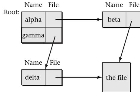
Figure 8.16: A file can have two different names, each in its own directory. In this example, the two pathnames `/alpha/beta` and `/gamma/delta` both lead to the same file.
