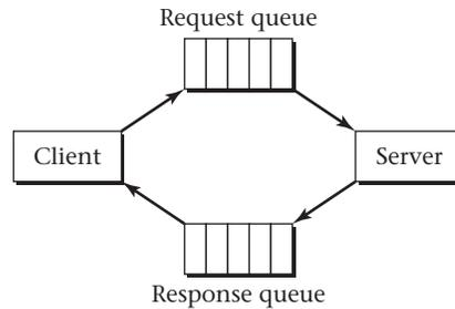
Figure 10.2: A client and server can engage in a request-response protocol using two message queues. Typically, the client tags each request message with a unique identifying string, known as a *correlation ID*. The server copies this ID into the resulting response message so that the client knows to which request the response corresponds.
