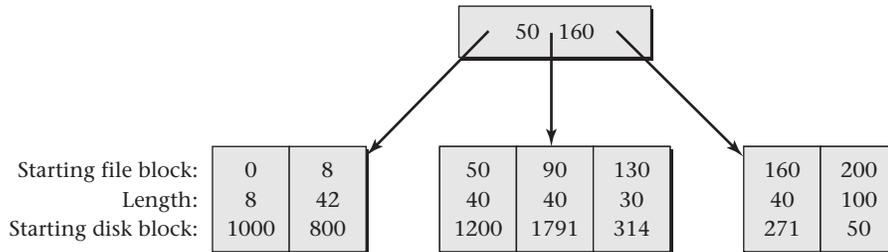
Figure 8.13: This small B<sup>+</sup>-tree extent map contains information that can be used to find each extent’s range of file block numbers and range of disk block numbers. Because the tree is a B<sup>+</sup>-tree rather than a B-tree, all the extents are described in the leaves, with the nonleaf node containing just navigational information.
