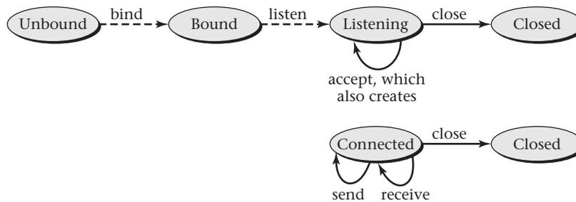
Figure 9.6: This state diagram shows the life cycle of server-side stream sockets used to accept TCP connections. In the Java API, the class `java.net.ServerSocket` is used for this purpose, and the bind and listen operations ordinarily are performed automatically as part of the constructor. Each time the accept operation succeeds, a new connected socket is returned, which in the Java API is an instance of `java.net.Socket`.
