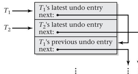
Figure 5.10: Rather than having a separate undo log for each transaction, the undo logs can be combined. In this case, the entries for any one transaction are chained together, as shown here, so that they can be efficiently processed as though in a separate log.
