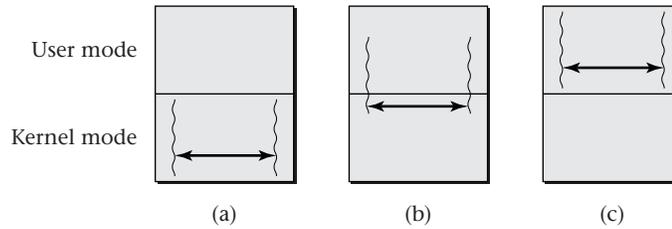
Figure 7.8: Three relationships are possible between threads, the scheduling and dispatching code that switches threads, and the operating modes: (a) the threads can be part of the kernel, along with the kernel’s scheduler and dispatcher; (b) the threads can run mostly in user mode, but be scheduled and dispatched in the kernel; (c) the threads can run in user mode along with a user-level scheduler and dispatcher.
